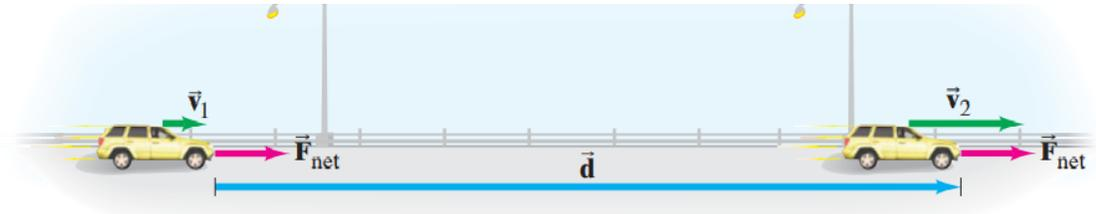
**FIGURE 6-7** A constant net force  $F_{\text{net}}$  accelerates a car from speed  $v_1$  to speed  $v_2$  over a displacement  $d$ . The net work done is  $W_{\text{net}} = F_{\text{net}}d$ .
