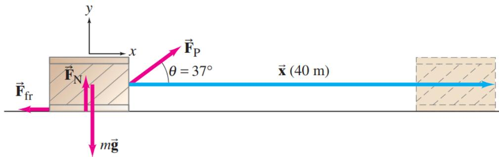
**EXAMPLE 6–1** **Work done on a crate.** A person pulls a 50-kg crate 40 m along a horizontal floor by a constant force  $F_P = 100$  N, which acts at a  $37^\circ$  angle as shown in Fig. 6–3. The floor is rough and exerts a friction force  $\vec{F}_{fr} = 50$  N. Determine (a) the work done by each force acting on the crate, and (b) the net work done on the crate.
