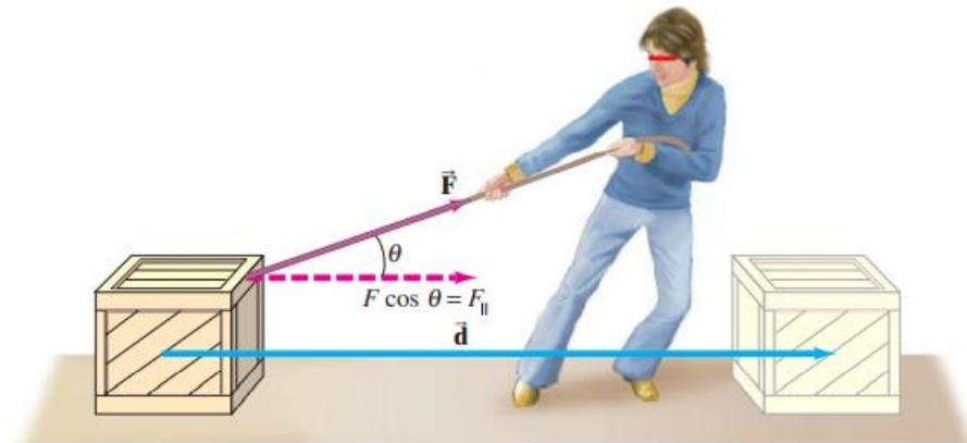
**FIGURE 6-1** A person pulling a crate along the floor. The work done by the force  $\vec{F}$  is  $W = Fd \cos \theta$ , where  $\vec{d}$  is the displacement.
