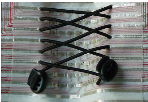
Fig. 9.10 Pocket version with elastic cords. This version allows the reader to see the conductive pads inside, while the elastic cords generate the pressure between textile and device
